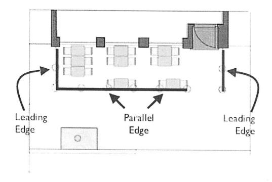
FIGURE 1 Illustration of leading edge and parallel edge of barrier
